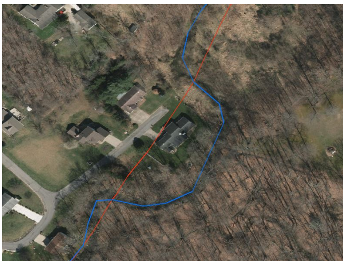
Figure 6: Example of modified stream cutting through a house in a section of Cheat watershed
