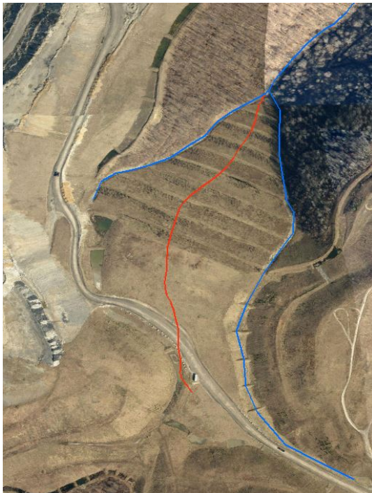
Figure 2: Example of modified stream segments in a surface mining area in a part of Coal watershed
