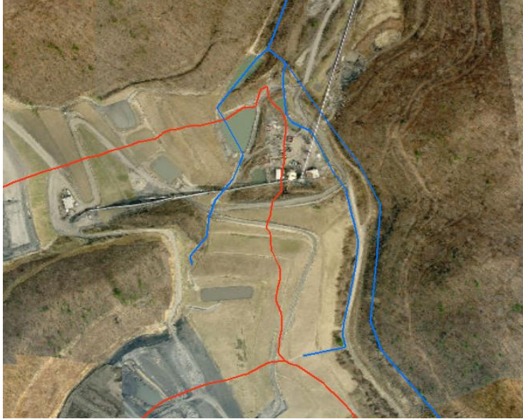
Figure 1: Example of deleted and modified stream segments in a part of Gauley watershed
