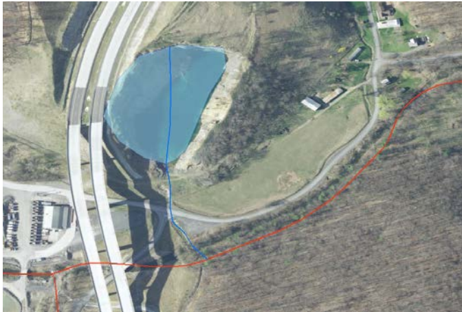
Figure 5: Example of an added stream segment and connected waterbody in a part of North Brach Potomac watershed
